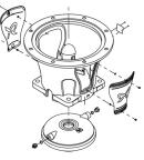
The pump is fitted with a balanced O-ring seal unit with a rigid torque-transmission system.
