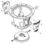
The pump is fitted with a balanced O-ring seal unit with a rigid torque-transmission system. This seal type is assembled in a cartridge unit which makes replacement safe and easy.
