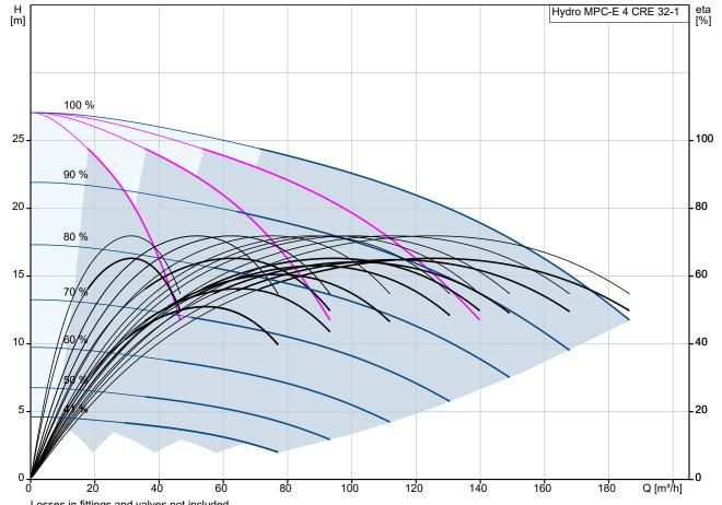
Losses in fittings and valves not included Pumped liquid = Water Liquid temperature during operation = 20  $^{\circ}$ C Density = 998.2 kg/m³
