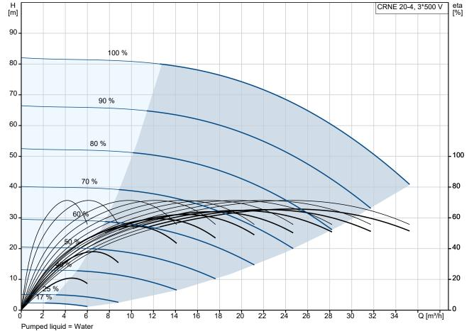
Liquid temperature during operation = 20 °C
