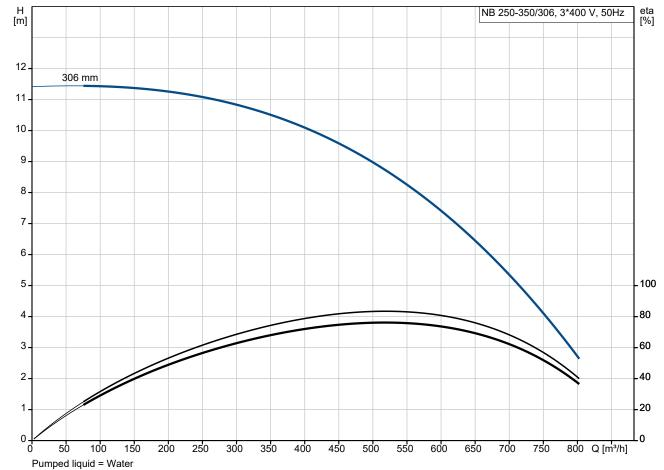
Liquid temperature during operation = 20 °C
