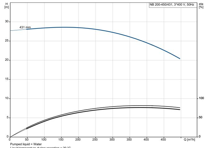
Liquid temperature during operation = 20 °C
