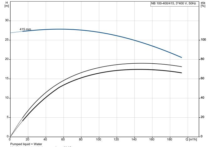
Liquid temperature during operation = 20 °C
