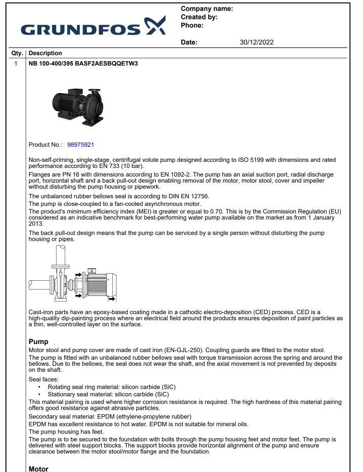
The motor is a totally enclosed, fan-cooled motor with principal dimensions to IEC and DIN standards. Electrical tolerances comply with IEC 60034.
