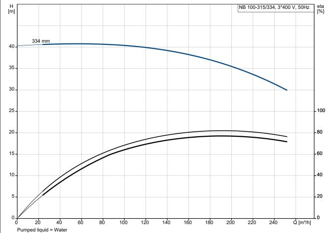
Liquid temperature during operation = 20 °C
