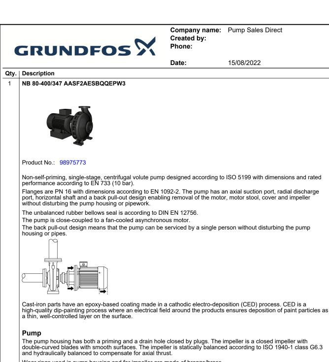
Wear rings used in pump housing and for impeller are made of bronze/brass. Motor stool and pump cover are made of cast iron (EN-GJL-250). Coupling guards are fitted to the motor stool. The pump cover is provided with a manual air vent screw for venting of the pump housing and the shaft seal chamber.
