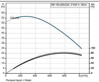
Liquid temperature during operation = 20 °C Density = 998.2 kg/m³
