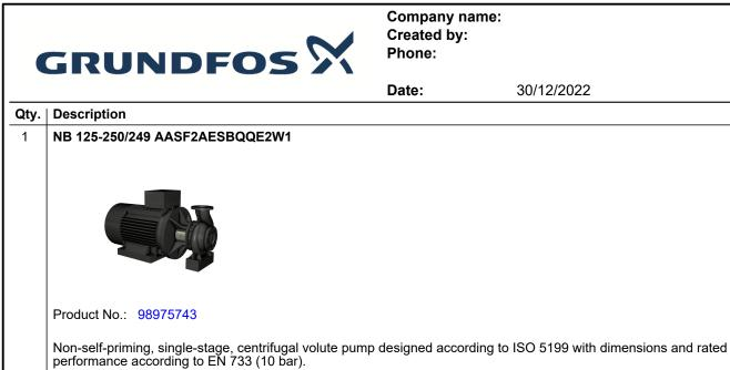
Flanges are PN 16 with dimensions according to EN 1092-2. The pump has an axial suction port, radial discharge
