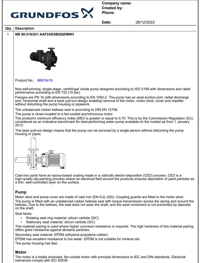
The motor efficiency is classified as IE3 in accordance with IEC 60034-30-1.
