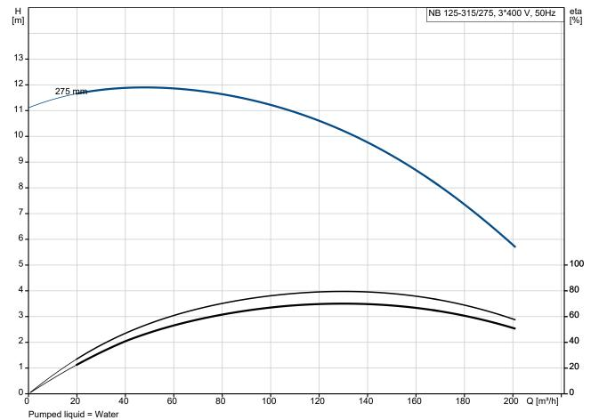
Liquid temperature during operation = 20 °C
