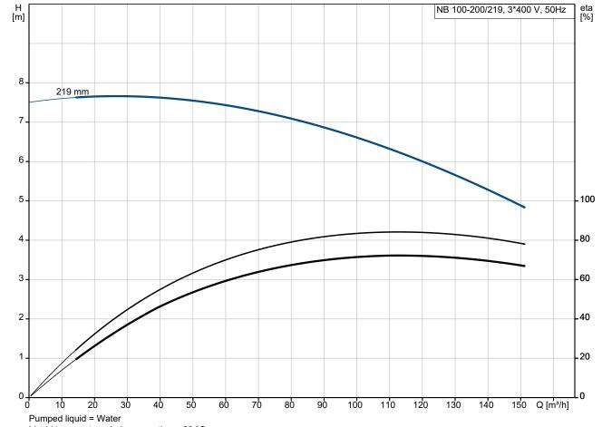
Liquid temperature during operation = 20 °C
