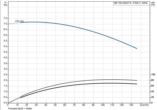
Liquid temperature during operation = 20 °C
