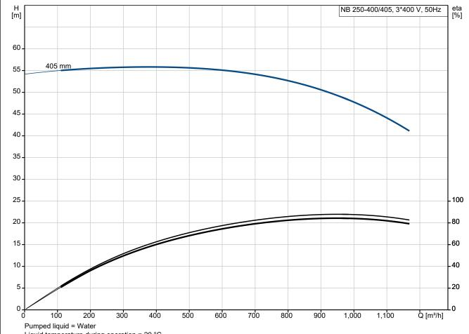
Liquid temperature during operation = 20 °C
