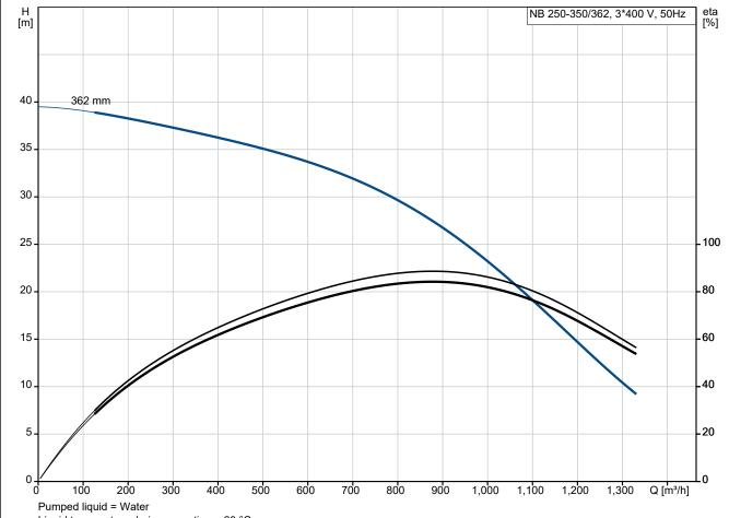
Liquid temperature during operation = 20 °C
