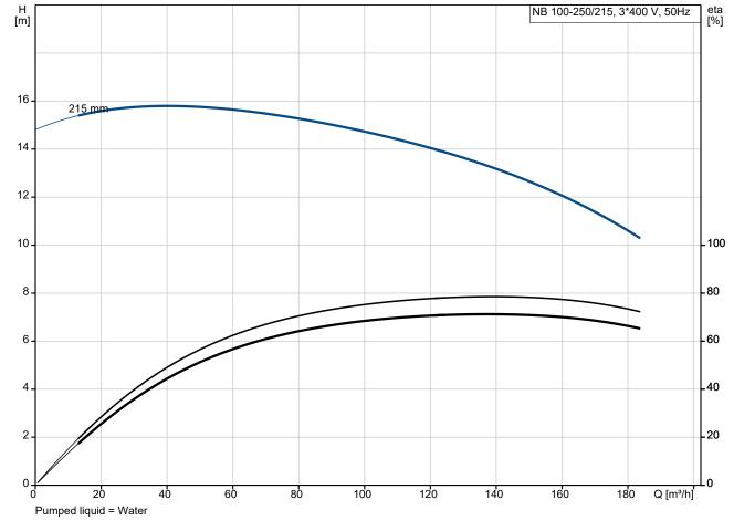
Liquid temperature during operation = 20 °C
