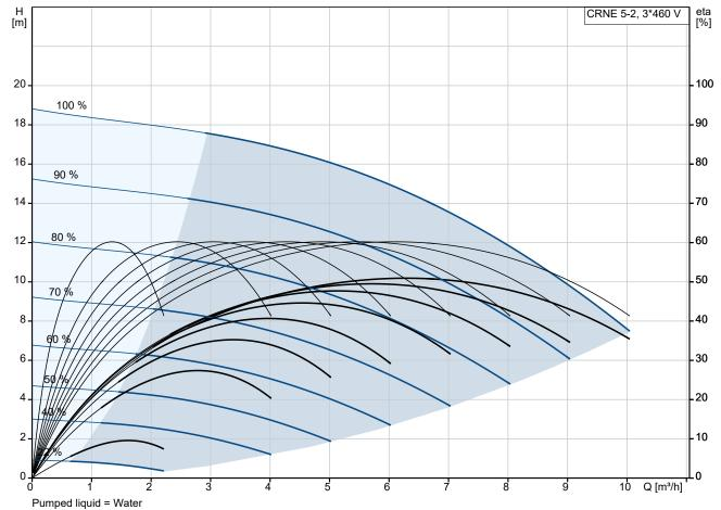
Liquid temperature during operation = 20 °C Density = 998.2 kg/m³
