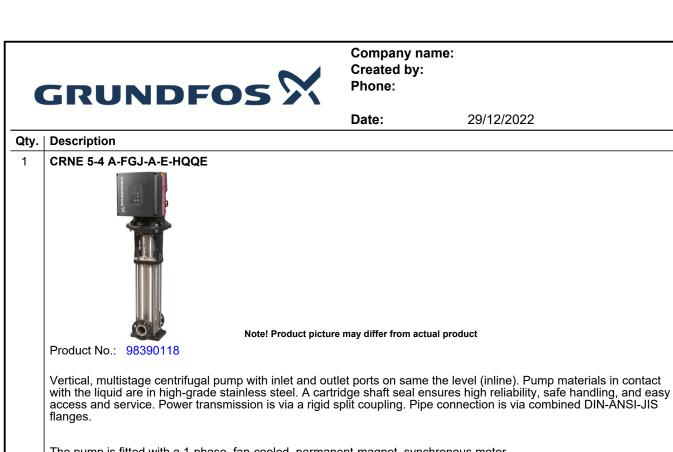
The pump is fitted with a 1-phase, fan-cooled, permanent-magnet, synchronous motor.
