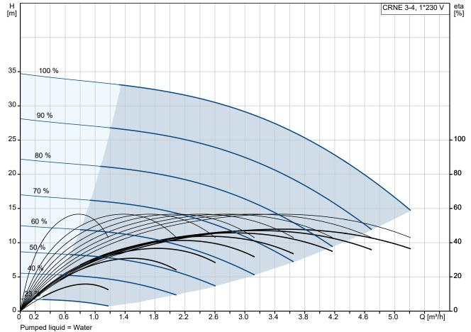
Liquid temperature during operation = 20 °C
