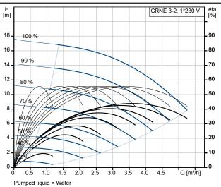
Liquid temperature during operation = 20 °C Density = 998.2 kg/m³
