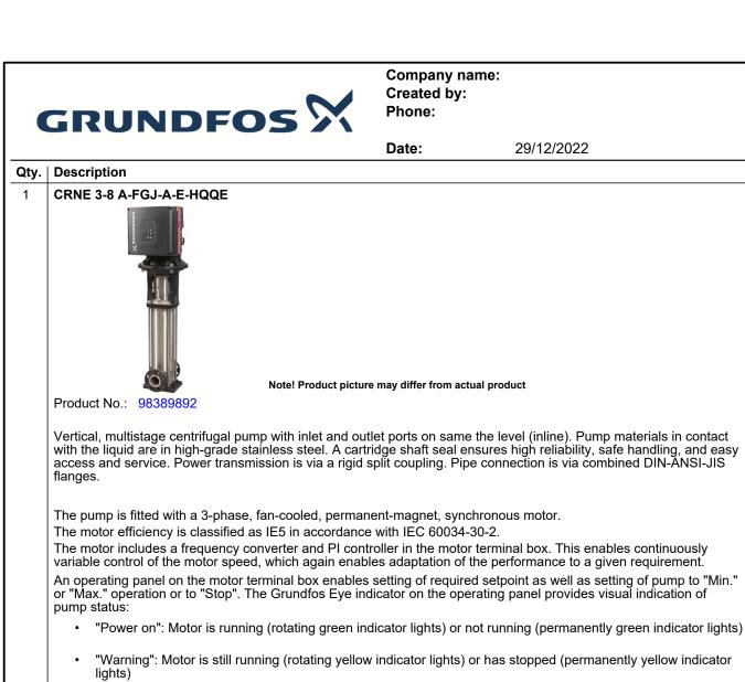
• "Alarm": Motor has stopped (flashing red indicator lights).
