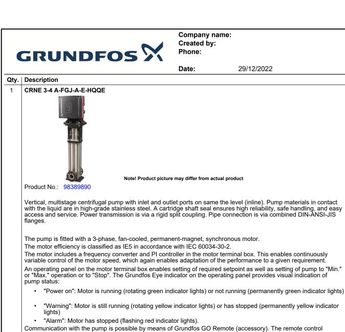
enables further settings as well as reading out of a number of parameters such as "Actual value", "Speed", "Power input" and total "Power consumption".
