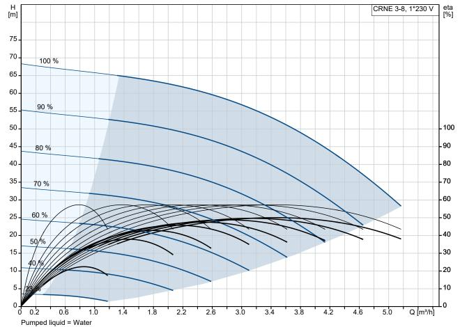
Liquid temperature during operation = 20 °C
