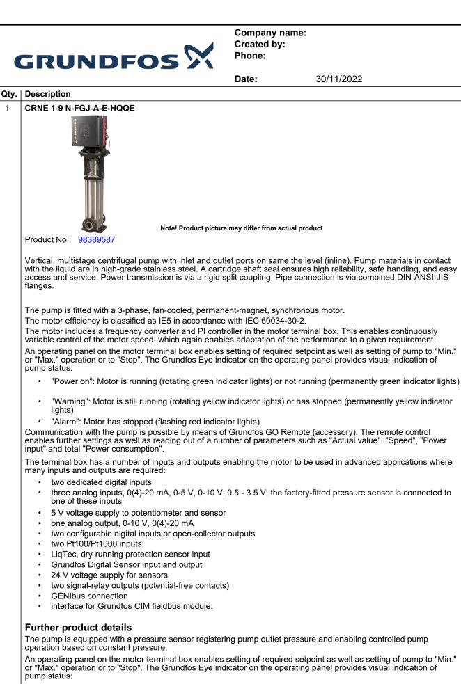
"Power on": Motor is running (rotating green indicator lights) or not running (permanently green indicator lights)
