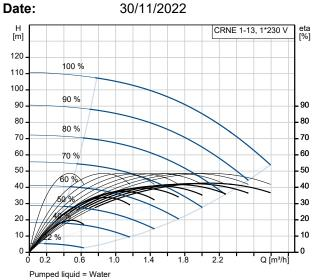
Liquid temperature during operation = 20 °C
