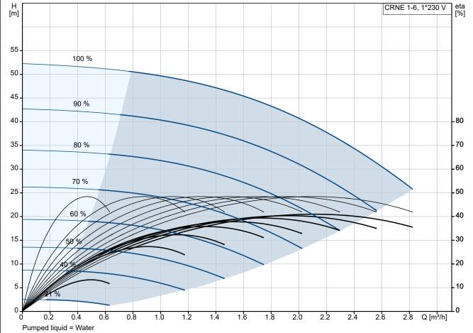
Liquid temperature during operation = 20 °C
