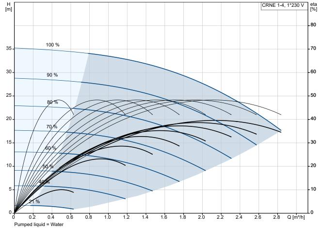
Liquid temperature during operation = 20 °C
