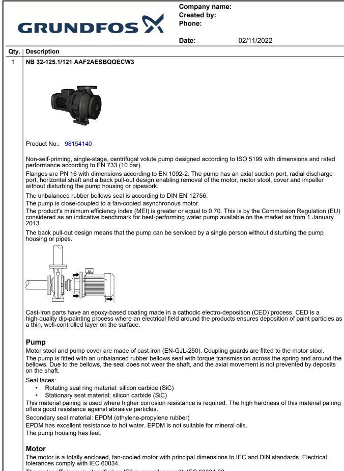
The motor efficiency is classified as IE2 in accordance with IEC 60034-30.
