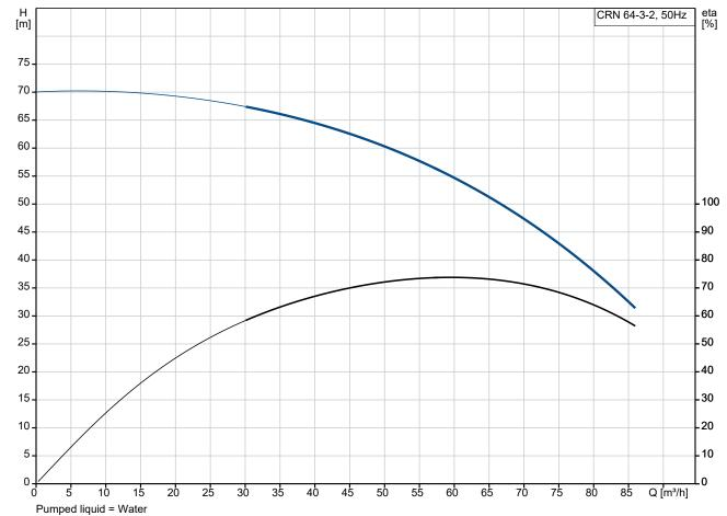
Liquid temperature during operation = 20 °C
