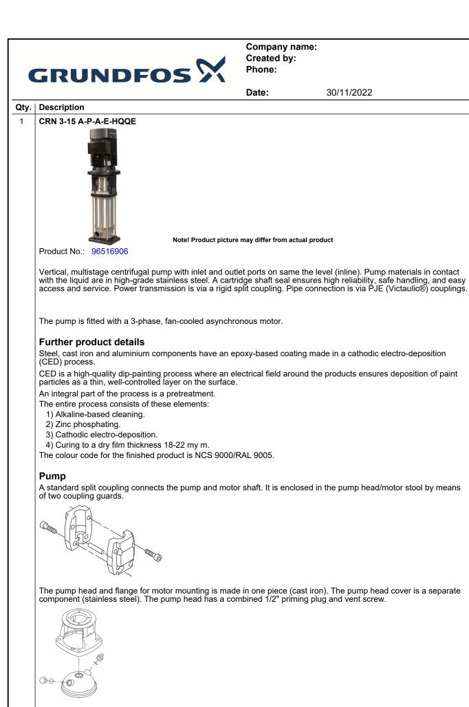
The pump is fitted with a balanced O-ring seal unit with a rigid torque-transmission system. This seal type is assembled in a cartridge unit which makes replacement safe and easy.
