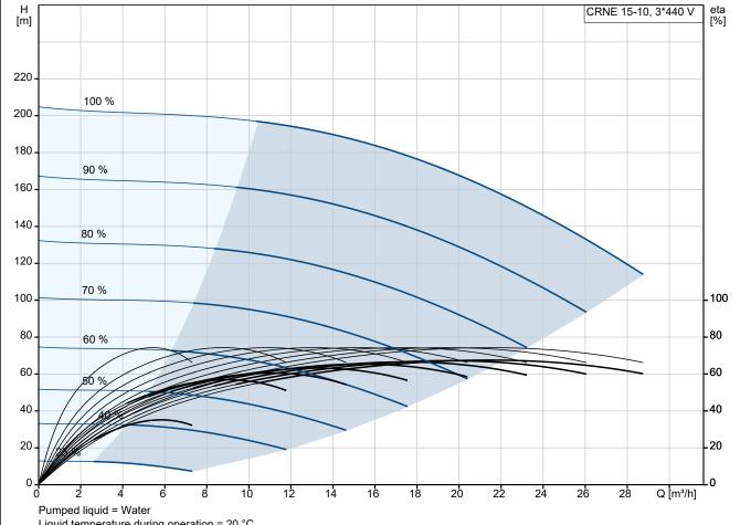
Liquid temperature during operation = 20 °C
