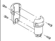
The pump head and flange for motor mounting is made in one piece (cast iron). The pump head cover is a separate component (stainless steel). The pump head has a combined 1/2" priming plug and vent screw.
