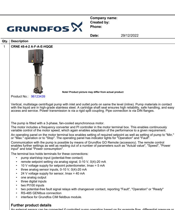
An external sensor can be connected if controlled pump operation based on for example flow, differential pressure or temperature is required.
