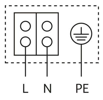
Blocking current-proof motor **Single-phase motor** (EM) 2-pole - 1~230 V, 50 Hz With built-in capacitor
